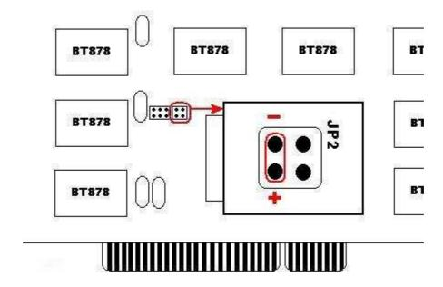
The other side of cable attaches on the M/B Reset, and please note the +/-poles.
