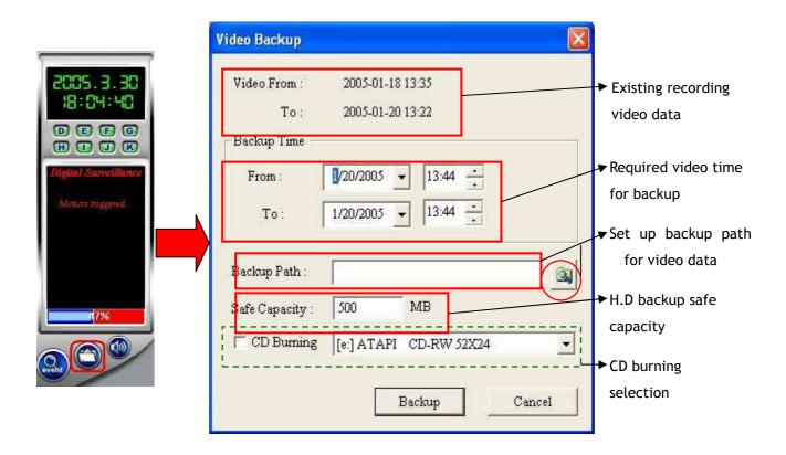
Please select the required video time for backup within the range of existing recording video data, input or select the backup path then click on "Backup" icon to perform backup instruction. (This method supports to backup in removable disk and network drive)
