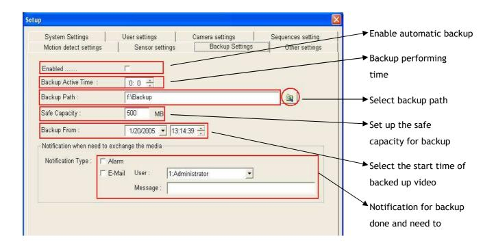
This method is to backup 24 hours recording data since the start of the required video automatically by setting up the performing time in advance and support to backup in host computer's hard disk drive only, network drive is not supported for backup.
